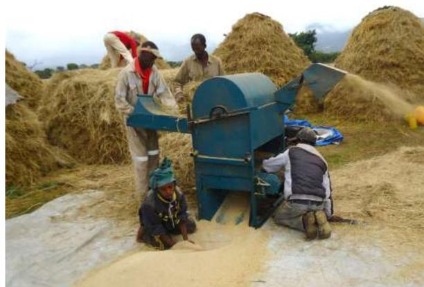
A typical teff threshing service provision using partial cleaning thresher
